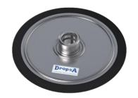
It is advisable to always use the follower plate, it is very important when the temperature is low and when high viscosity grease is used. Because of the depression created by the pump, the plate is attracted towards the bottom of the drum by atmospheric pressure. It pushes the grease into the pump and avoids air cavities. It also removes the grease remaining on the walls, down to the bottom of the drums.
