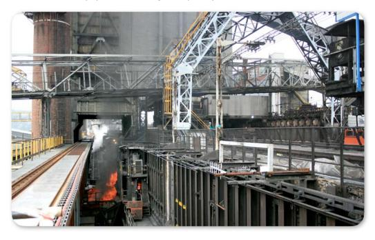
Coke oven are used to turn coal into coke. The process is done by the charge car loading the coal into the oven. After the coal has been heated to high temperatures the pusher car dislodges the coal into the transfer car.
