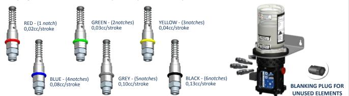
...There are 6 different pump element sizes for you to select from and they are ordered separately from the pump according to how many lubrication points need to be serviced.
