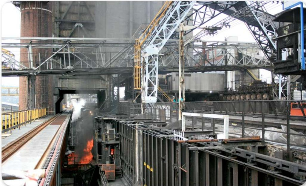
Coke oven are used to turn coal into coke. The process is done by the charge car loading the coal into the oven. After the coal has been heated to high temperatures the pusher car dislodges the coal into the transfer car.
