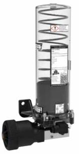
The Locopump S3 grease is an ideal single acting pneumatic grease pump generally used in single line progressive divider lubrication systems. The transparent reservoir allows the user to clearly see the quantity of grease remaining and a low level grease switch is present to provide remote alarm signals to the machine it is mounted on. Additionally, the reservoir lid can be modified to install a High level or a Dropsa continual level sensing device.
