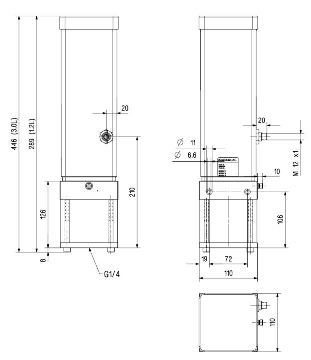
Figure 3: Single Piston Pump AM with float switch
