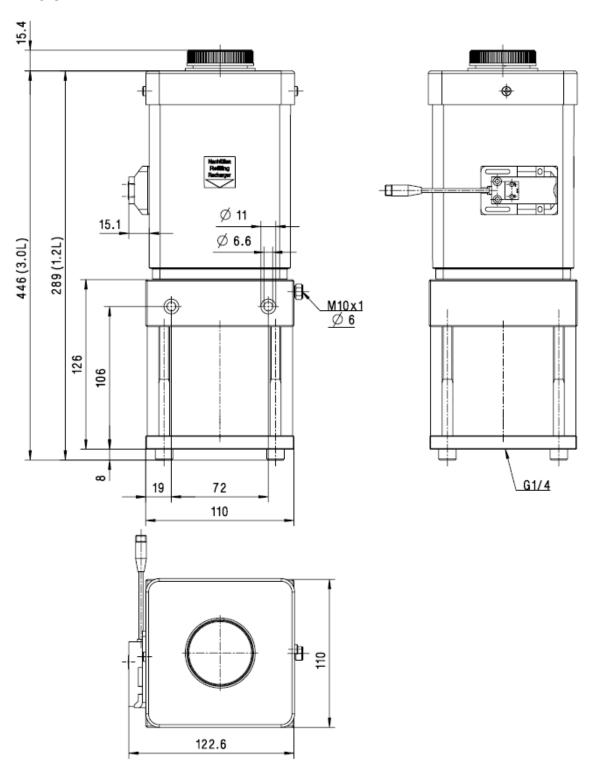
Figure 2: Single Piston Pump AM with capacitive level control
