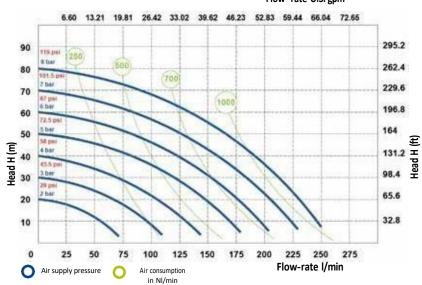
The curves and performance values refer to pumps with submerged suction and a free delivery outlet with water at  $20^{\circ}$ C and vary according to the construction material.
