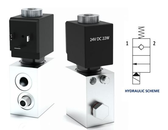
The **EV-2 SHUT-OFF** valves consist of a **"NC"** 2-way solenoid valve and an aluminium body to be applied directly on the inlet of progressive dividers.
