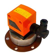
The laser probe possesses a representative and programming display mounted on board. It is possible to operate in analogue mode (with signal from 4 to 20 mA) or in digital mode (two outputs and four intervention thresholds).
