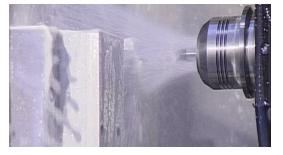
With **External** Lubrication: oil is transported via a nozzle to the cutting surface. Dropsa has a complete product line from simple, easy to install products such as the **Grip** and **Vip4Tools** series for External lubrication (please ask for documentation).
