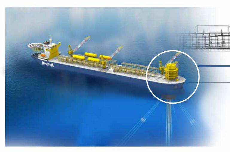
The **FPSO** turret let the vessel rotate up to 360° around the pivoting point.
