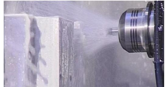
With **External** Lubrication: oil is transported via a nozzle to the cutting surface. Dropsa has a complete product line from simple, easy to install products such as the **Grip** and **Vip4Tools** series for External lubrication (please ask for documentation).
