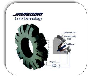
Magnom™ core elements are comprised of an annular magnet and two innovatively formed steel plates. The steel plates direct the lubricant flow and magnetic flux through channels designed to bring all the ferrous contaminants in the lubricant within the range of the magnets.
