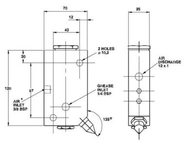
\* RATIO 8:1 AIR PRESSURE 3 BAR MIN. 12 BAR MAX.
