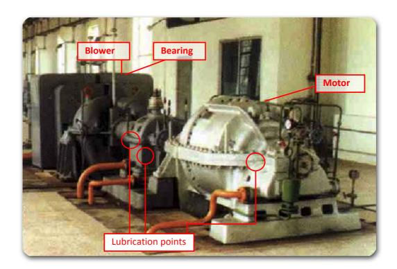
The diagram on the right represents a common lubrication arrangement for a blower.
