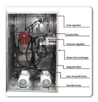
Below is an example of an API Unit for a Fertisiler Plant
