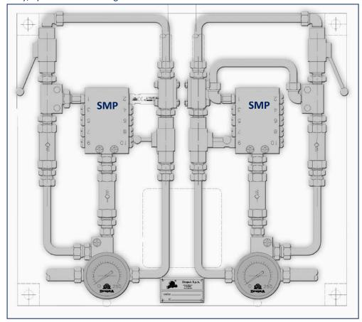
The SMP units are fitting with the latest Dropsa Ultrasensor spool sensor product: a revolutionary patented system that has no moving parts and made in AISI 316 Stainless Steel.
