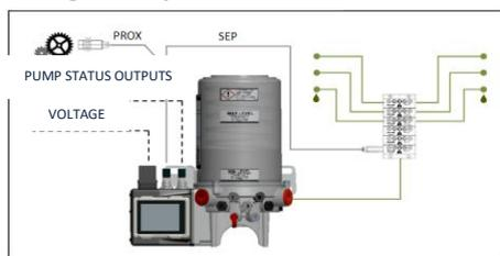
With this configuration, the lubrication phase is formed of a **single cycle** (Number of cycles: 1) that starts **every 2 pulse signals** (Interval Pulses: 2) arriving **on Input 1** (Input 1: Pulses Count). The lubricating phase finishes with the transition 0 → 1 → 0 (or 1 → 0 → 1) on Input 2 (Input 2: SEP/PROX), which must occur within 30 seconds of the start of the lubrication cycle (Cycle Timeout: 30s). Otherwise, a cycle alarm is generated.
