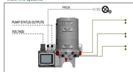
With this configuration, the lubrication phase is formed of a **single cycle** (Number of cycles: 1) that starts **every 6m 00s** (Interval Time: 6m 00s) or **every 10 pulse signals** (Interval Pulses: 10) arriving on Input 1 (Input 1: Pulses Count). The lubrication phase finishes on the achievement of 2 complete revolutions of the pump motor (Cycle Rotations/Pulses: 2).
