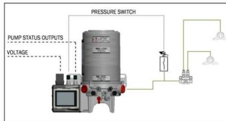
With this configuration, the lubrication phase is formed of a **single cycle** (Number of cycles: 1) that starts **every 6m 00s** (Interval Time: 6m 00s) and finishes once the **line pressure** is reached, which must occur within 30 seconds of the start of the lubrication cycle (Cycle Timeout: 30s). Otherwise, a cycle alarm is generated.
