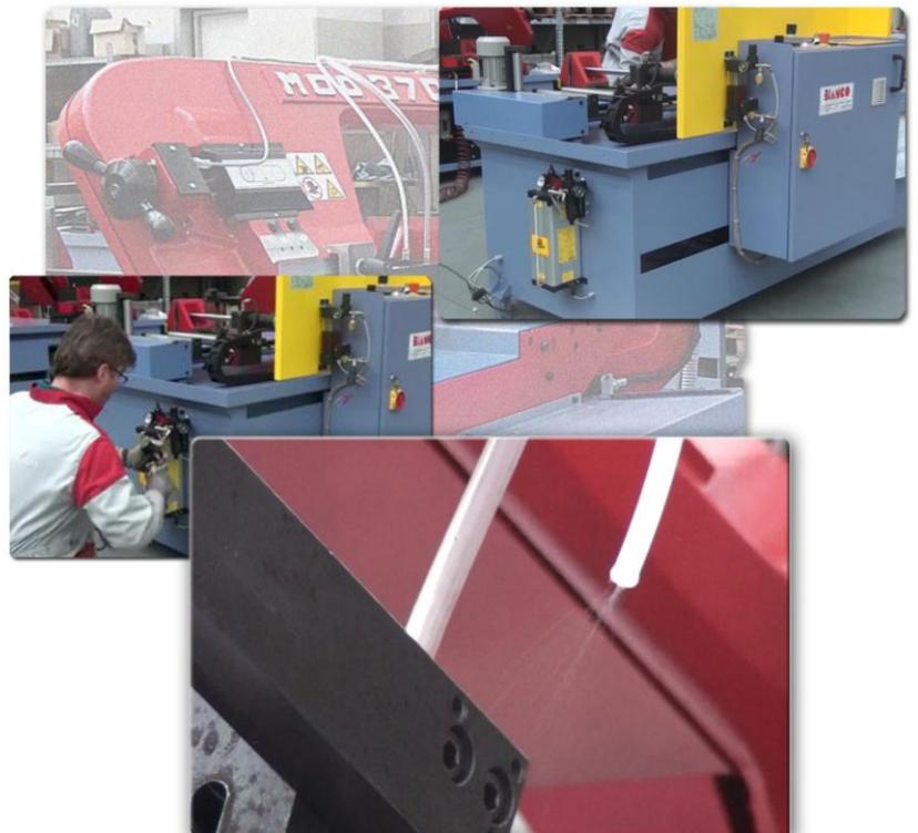
In addition **Miquel modular system** increase the life of the tool (thanks to the reduction of friction between tool and work piece and the heat removal on the machining) involves a minimal use of biodegradable oils, **eliminating** the **problems** associated with disposal of the **emulsions** and also **reducing the environmental impact**.
